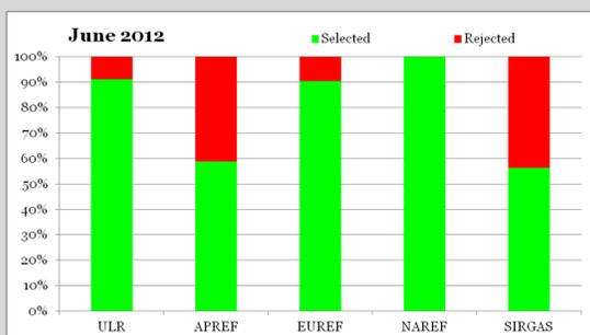
Figure 2: Level of agreement of ULR, APREF, EUREF, NAREF and SIRGAS solutions wrt ITRF2008
